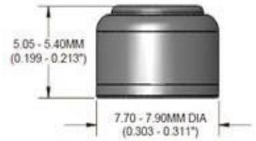
DIMENSIONS SHOWN ARE IEC STANDARDS FOR ENGINEERING TOLERANCES CONTACT RAYOVAC.
